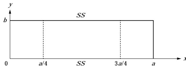
Figure 2. Three-span continuous rectangular plates in one direction.
